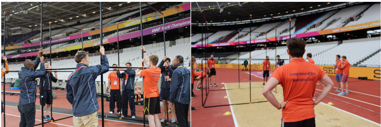
Figure 2. The calibration frame was constructed and filmed before and after the competition.
