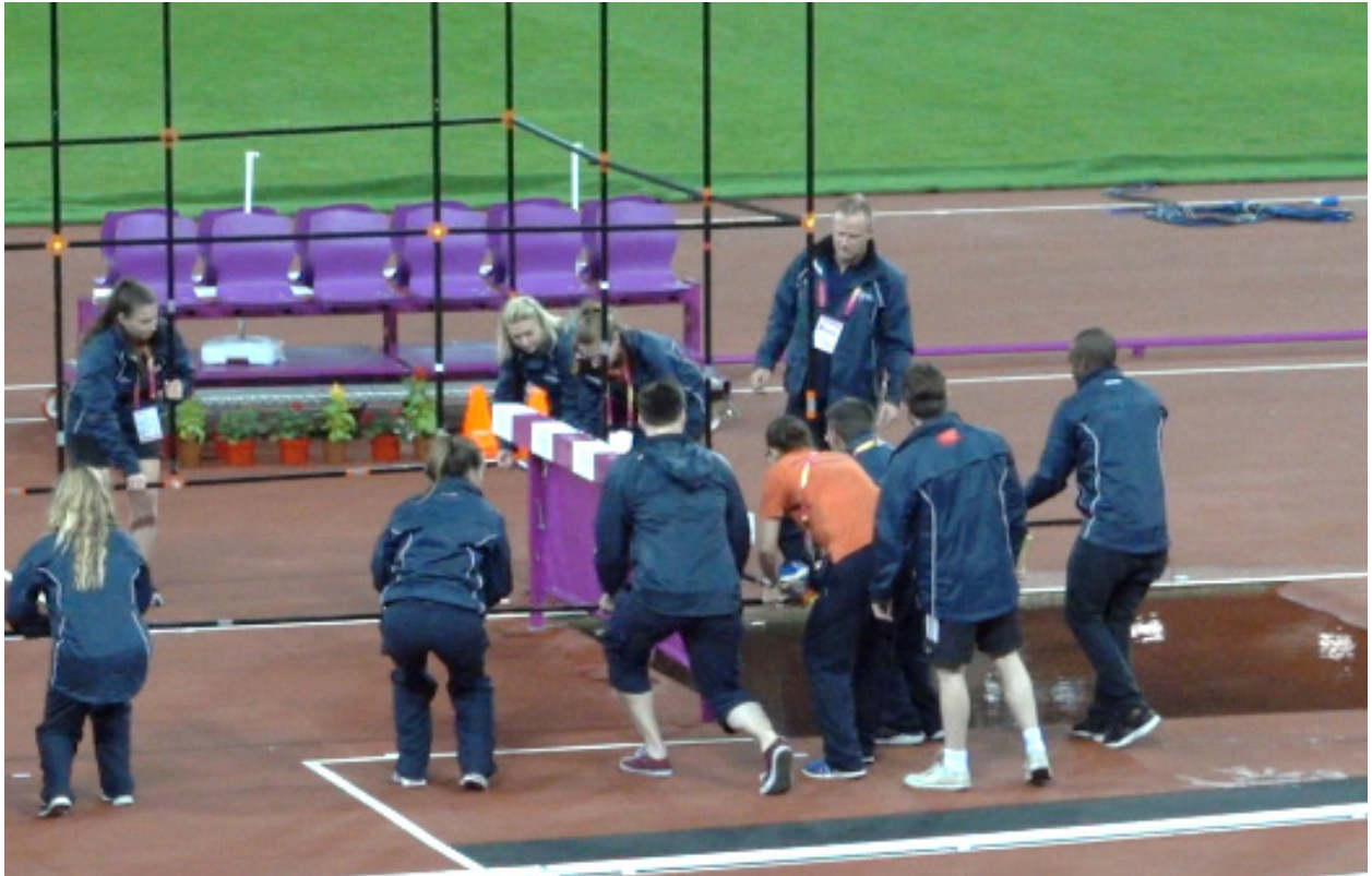
Figure 2. The calibration frame was constructed and filmed before and after the competition.
