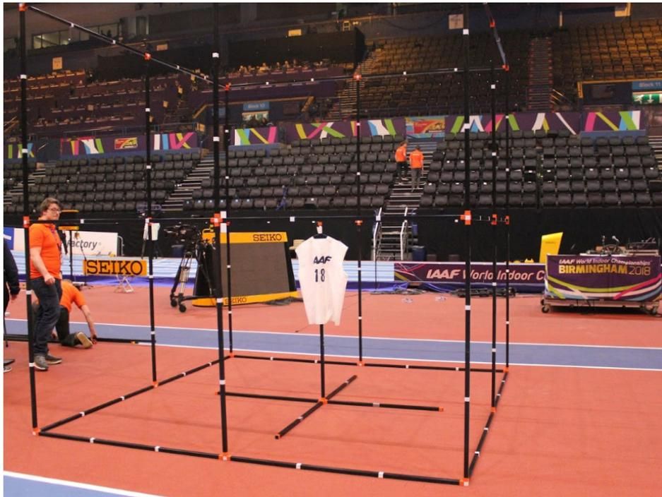
Figure 2. The calibration frame was constructed and recorded before and after the competition.
